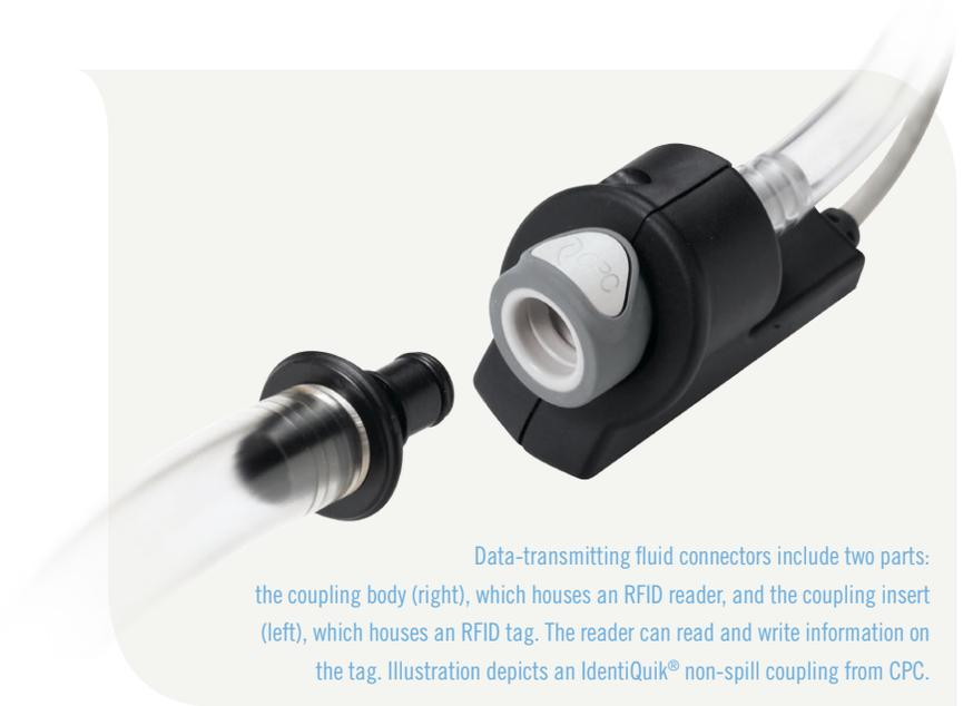
Data-transmitting fluid connectors include two parts: the coupling body (right), which houses an RFID reader, and the coupling insert (left), which houses an RFID tag. The reader can read and write information on the tag. Illustration depicts an IdentiQuik® non-spill coupling from CPC.
