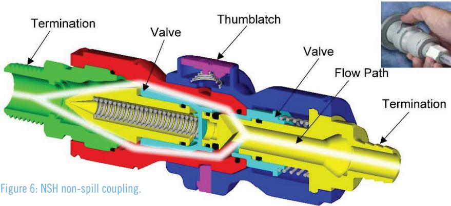
Figure 6: NSH non-spill coupling.
